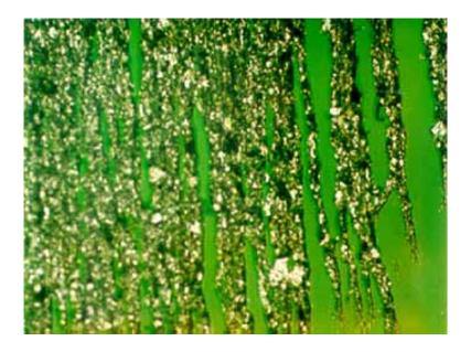
**An analytical ferrogram** at 200X magnification reveals an abnormal quantity of combined rolling and sliding wear particles indicating abnormal gear wear in the system.
